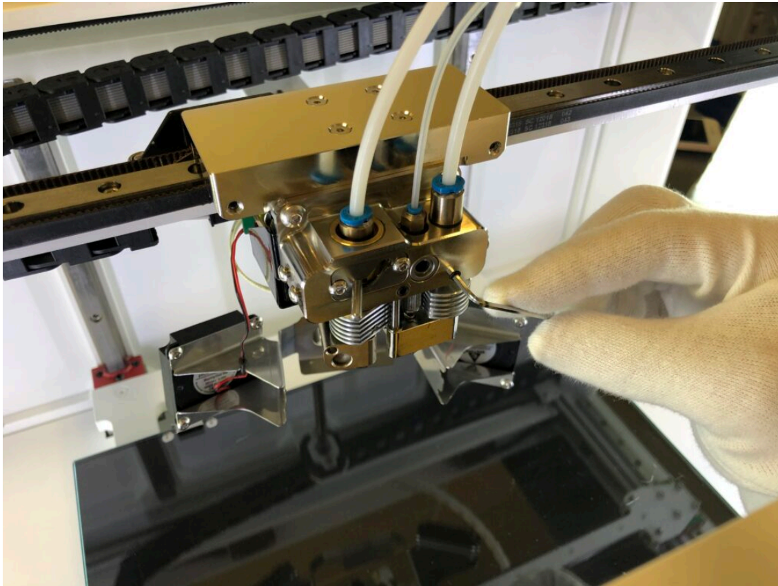
4. Using the wrench key or pliers unscrew the fiber guiding bushing.
